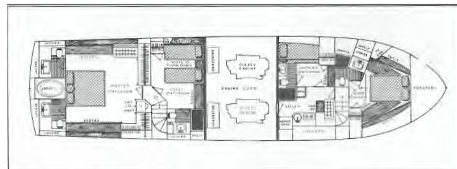
Both the owner's stateroom and engine room are full-beam.
